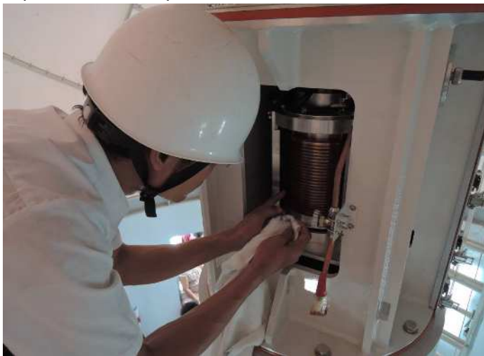
Clean the slip ring with dry soft cloth.
