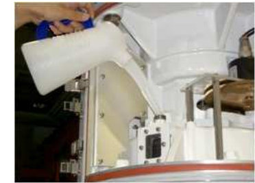
Reduction gear oil replacement
